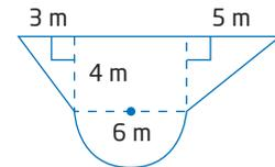
The patio area will be made of interlocking paving stones with different stones along the border. The paving stones cost  $\$52.95/\text{m}^2$ . The border stones are priced according to the length of the border and cost  $\$15.50/\text{m}$ . How much will the materials for the patio cost, including 8% PST and 7% GST? Allow an additional 10% to account for stones that must be cut for the design.
