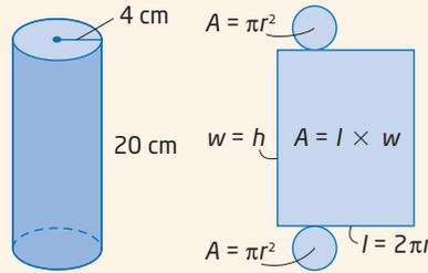
The surface area of the cylinder consists of the top and bottom, which are circles, and the curved surface, which is a rectangle.
